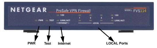
Figure 2-1: FVS114 front panel
